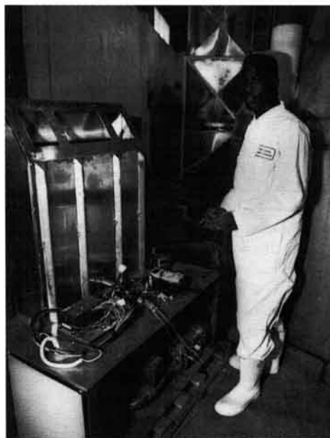
Zikomo constructed all their own equipment, including this keg washing machine.
